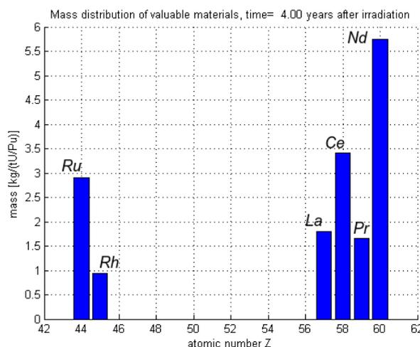
Figure 1: Mass distribution of valuable materials in kg per tonne of heavy metal fuel
